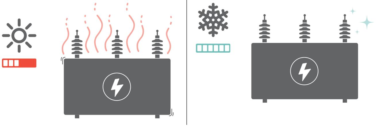
temperature climates could cause significant damage to the networks.<sup>42</sup> With lower outside temperatures, transformers can tolerate higher loads for longer time periods than when external temperatures are higher which make transformers more likely to overheat. For many public power utilities, the concerns of the potential impacts on transmission
